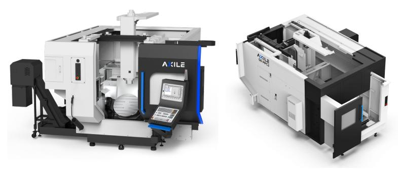
With a rotary table diameter of 600 mm the G6 is a compact vertical machining center designed for agile, smart machining of smaller workpieces requiring complex geometries and intricate features. This highly versatile VMC delivers full 5-axis CNC machining with the built-in spindle moving along the X/Y/Z-axes and the table moving in the rotary C-axis and the swiveling A-axis.
