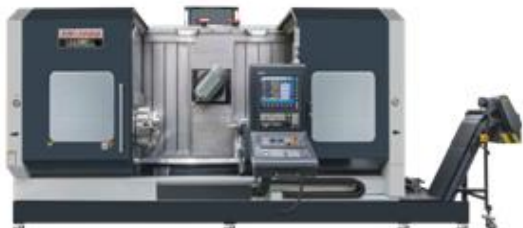
LEADWELL TASK MASTER TM-1500 CNC 5-AXIS simultaneous multi task Machine Tuning Spindle with C-axis: 1500RPM; 50 hp; 20" Hydraulic chuck; 7" bar capacity Milling Spindle with B axis: 12,000rpm; 35HP; B-axis: -10°/+230° Dual Automatic Tool Changers: Main ATC with 60 tools; 2nd ATC with 20"-long boring bar
