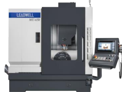
LEADWEL MU-650 TRAVEL COLUMN 5 AXIS 12000 RPM spindle X/Y/Z 620/520/460mm Table 650mm Dia. Tilt range +110 to -50 degrees 30 tool ATC
