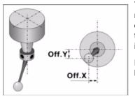
The cycle measures the deviation of the probe ball with respect to the tool-holder axis and the electronic radius of the probe. The electronic radius is the deflection of the probe since it makes contact until the probing signal is activated.
