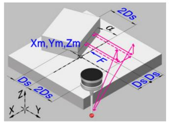
This cycle calculates the angle of the part with respect to the abscissa axis. This cycle may be used to measure angles between  $\pm 45^{\circ}$ .
