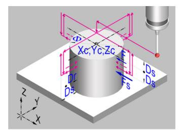
This cycle calculates the diameter of a boss and the real position of the center.
