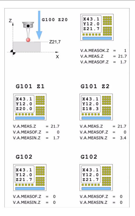
G101/G102. Include/exclude the measuring error in the theoretical coordinate.
