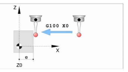
After probing, the CNC assumes the current axis position as the theoretical position. Functions G101 and G102 determine whether to consider or ignore the measuring error when updating the theoretical coordinate.
