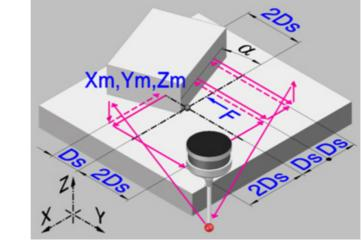
This cycle calculates the position of an outside corner and the angle of the part with respect to the abscissa axis. This cycle may be used to measure angles between  $\pm 45^{\circ}$ .
