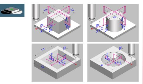
This cycle may be used to calculate the center of a rectangular or circular part or pocket of known dimensions as well as, in rectangular parts, the inclination of the part with respect to the abscissa axis.
