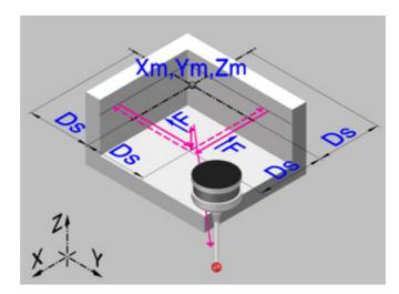
This cycle calculates the position of an inside corner.
