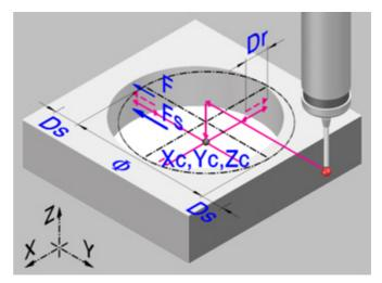
This cycle calculates the diameter of a hole and the real position of the center.
