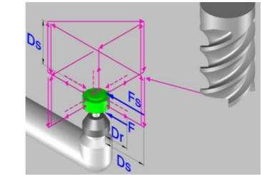
This cycle may be used to calibrate a tabletop probe using a tool that has been calibrated in radius and length.
