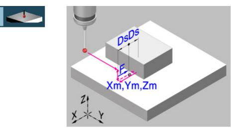
This cycle measures the part along the selected axis. With this cycle, it is also possible to correct the value of the wear of the tool used to machine the surface. The wear correction only takes place when the measuring error exceeds a programmed value.
