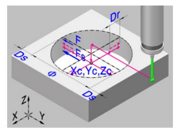
This cycle may be used to calibrate the probe located in the spindle. This probe will be the one used in the tool calibration canned cycles.
