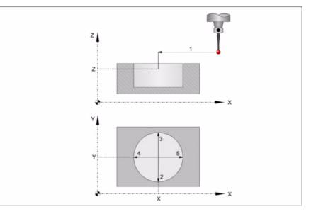
1 If the approach coordinates X Y Z have been programmed, approach movement. Probe's rapid movement (G00) from the cycle calling point to the center of the hole.
