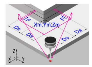
This cycle calculates the position of an outside corner.
