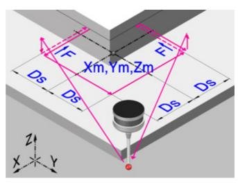
This cycle calculates the position of an outside corner.
