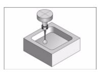
The probe must be placed within the pocket before calling the cycle.
