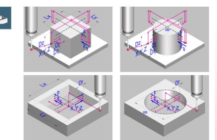
This cycle may be used to calculate the center of a rectangular or circular part or pocket of known dimensions as well as, in rectangular parts, the inclination of the part with respect to the abscissa axis.
