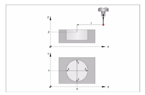
1 If the approach coordinates Xc Yc Zc have been programmed, approach movement. Probe's rapid movement (G00) from the cycle calling point to the center of the hole.
