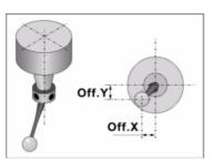
The cycle measures the deviation of the probe ball with respect to the tool-holder axis and the electronic radius of the probe. The electronic radius is the deflection of the probe since it makes contact until the probing signal is activated.
