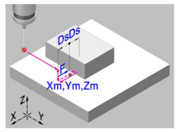
This cycle measures the part along the selected axis. With this cycle, it is also possible to correct the value of the wear of the tool used to machine the surface. The wear correction only takes place when the measuring error exceeds a programmed value.
