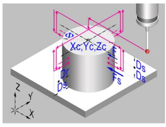
This cycle calculates the diameter of a boss and the real position of the center.
