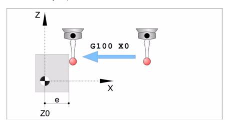
After probing, the CNC assumes the current axis position as the theoretical position. Functions G101 and G102 determine whether to consider or ignore the measuring error when updating the theoretical coordinate.
