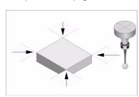
Depending on the part corner to be measured, the probe must be placed in the corresponding shaded area (see figure) before calling the cycle.
