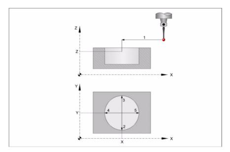
1 If the approach coordinates XYZ have been programmed, approach movement. Probe's rapid movement (G00) from the cycle calling point to the center of the hole.
