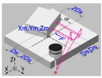
This cycle calculates the angle of the part with respect to the abscissa axis. This cycle may be used to measure angles between ±45°.
