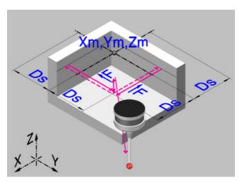
This cycle calculates the position of an inside corner.
