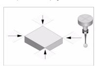
Depending on the corner of the part it is required to measure, the probe must be placed in the corresponding shaded area (see figure) before calling the cycle.
