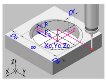
This cycle calculates the diameter of a hole and the real position of the center.
