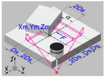
This cycle calculates the position of an outside corner and the angle of the part with respect to the abscissa axis. This cycle may be used to measure angles between ±45°.
