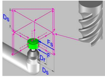
This cycle may be used to calibrate a tabletop probe using a tool that has been calibrated in radius and length.
