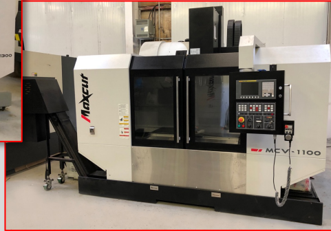
MCV-1100 with CAT#40 44" x 25" x 24" X/Y/Z-axis
