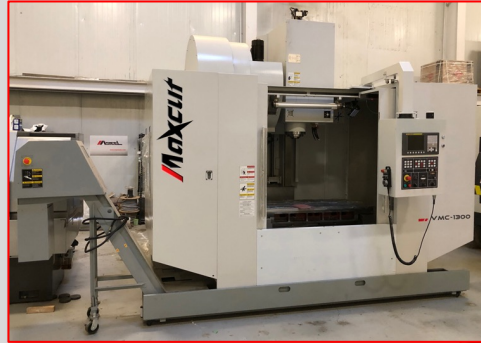
VMC-1300 with CAT#50 51" x 28" x 28" X/Y/Z-axis
