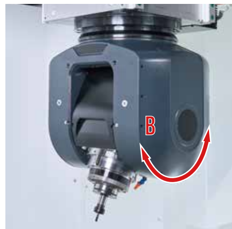
Swivelling B-axis head
